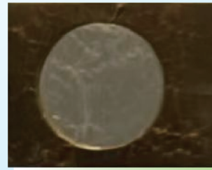
Nanometer-thick self-supporting ^{11}\text{B} target with \phi = 10.0 mm
