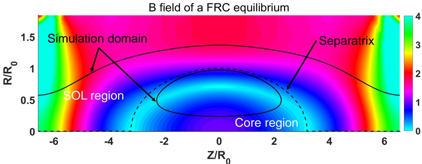
We simulate the above two flux surfaces use 1D model, with typical FRC Core and SOL parameters.
