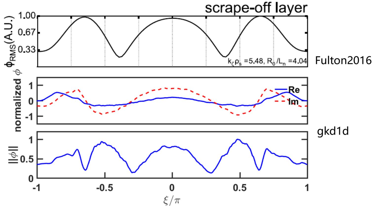
For both the real and the imaginary parts of  $\phi$ , the qualitative features are in agreement with Fulton 2016. However, the RMS value shows an additional feature, probably due to the interference between the real part and the imaginary part. More comparison and analysis need to be done.
