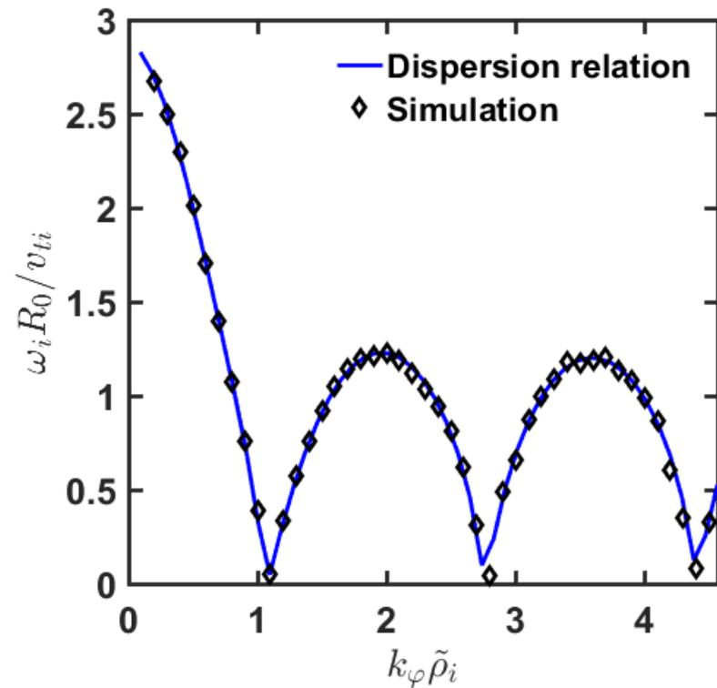
Benchmark tests of Program gkd1d at slab limit show good agreement with 0D theoretical DR results (error < 1%).
