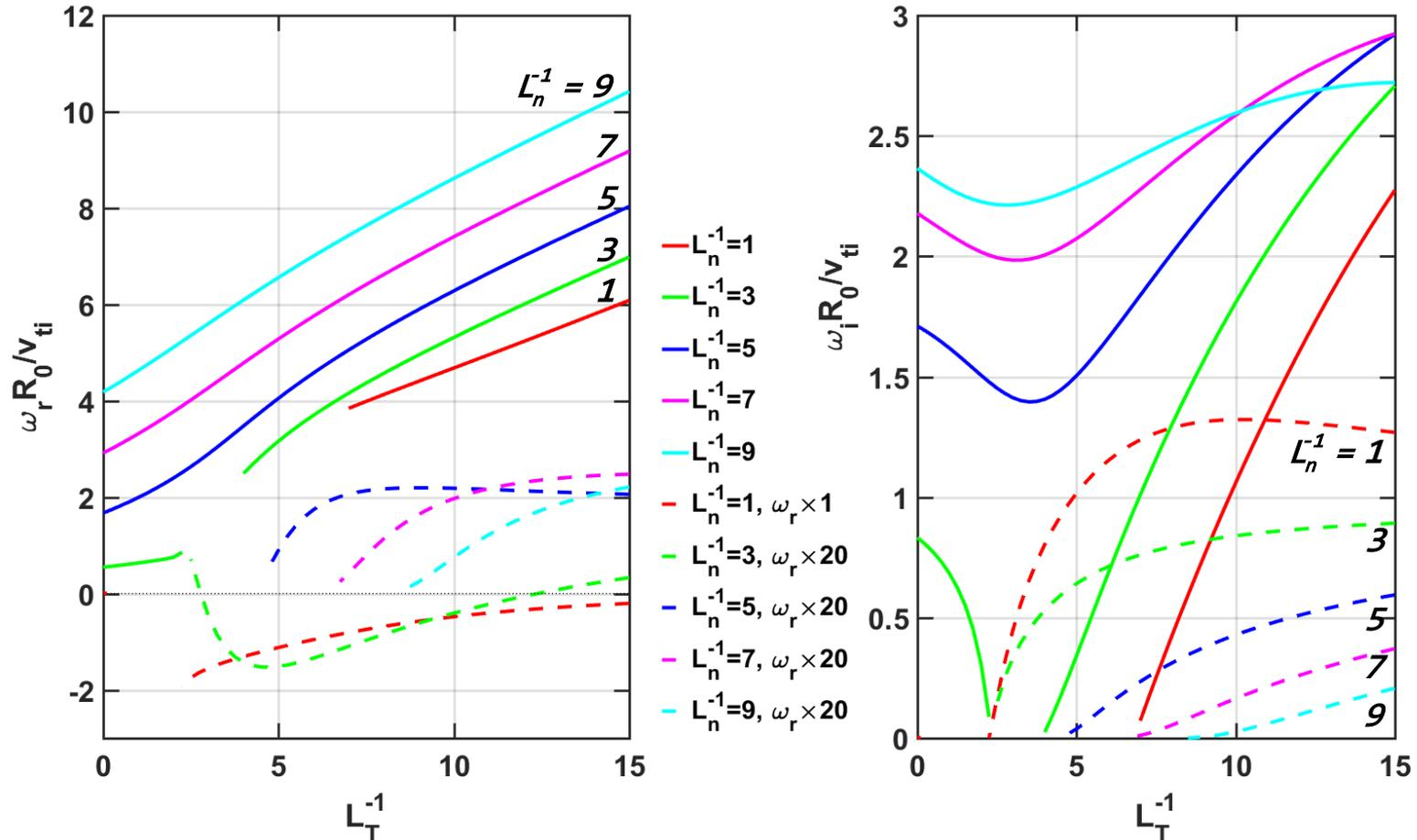
Two unstable branches. Increase of temperature gradient leads to the growth rate increase of linear drift instability.
